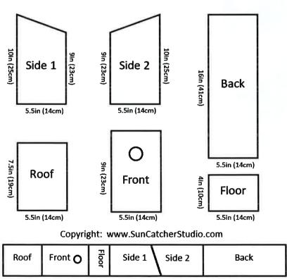
Use a single 1 x 6 board. The actual dimensions will be 3/4 inch thick and 5.5 inches wide. This project will require a board approximately 60" (1.5m) in length.
